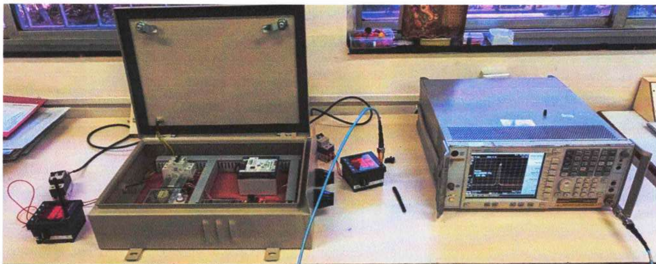
Measurement Setup for Conducted Emission
